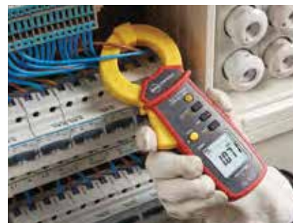
Differential current measurement with leakage current clamp
