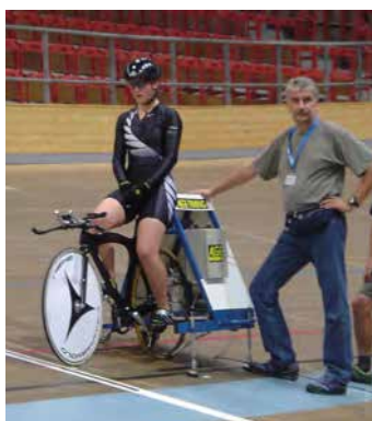
bicycle is held on the saddle and the rear wheel, as well as supported by the rear wheel
