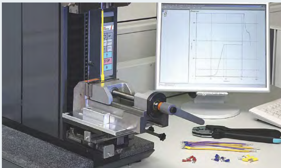
Conductor pull-out test
