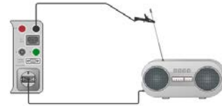
Insulation resistance test for Class II device
