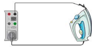
Substitute leakage test for Class I device
